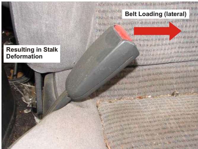
3. Seatbelt buckle stalk is deformed due to loading.
