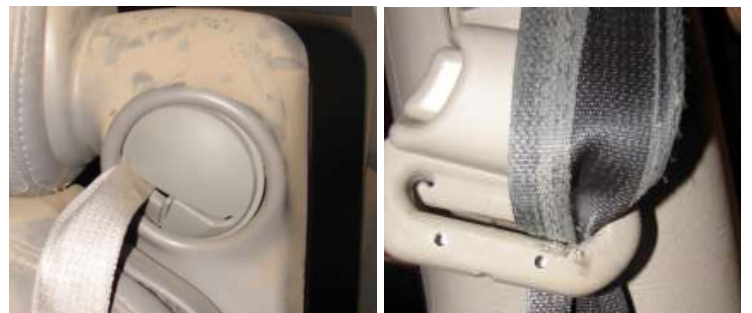
6. Webbing trapped in ABTS outlet / D-ring.
