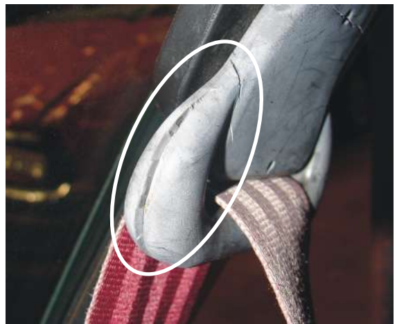
5. D-ring fractured due to loading.
