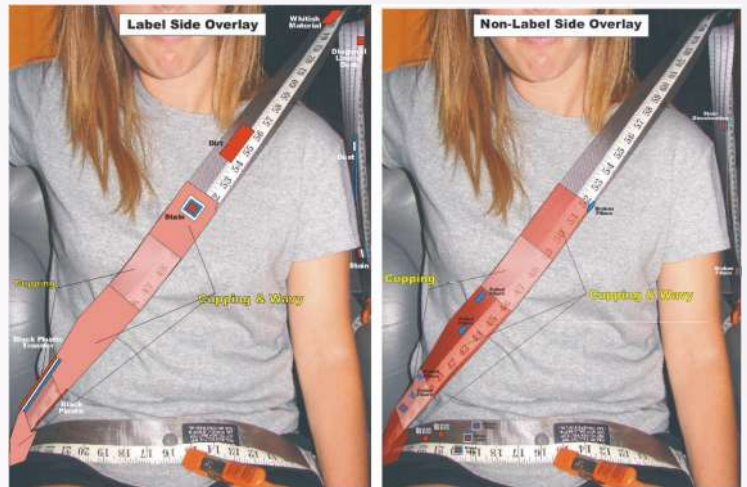
Example webbing inspection. Clothing fiber that is matched to Decedent's clothing found below "stowed belt" line.
